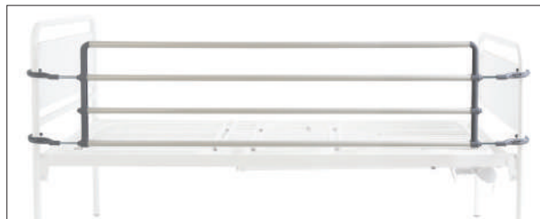
Cod. MP181 White painted steel reversible bedside rails Bedrail length 170 cm , total length 195 cm , maximum extension length 222 cm , hooking maximum length 210 cm , Ø 2,5 cm , bedside rail height 43cm
