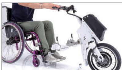
Push down (B) and hook Tiboda® through the ultra fast hooking system (C)
